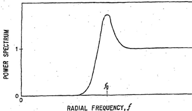
'310 patent fig.1. The horizontal axis represents the radial frequency, which is the reciprocal of the average spacing between the dots in the dot profile. A blue noise power spectrum has negligible frequency components below the principal frequency and high frequency components above the principal frequency. The principal frequency,  $f_g$ , varies from one gray level  $g$  to another:
